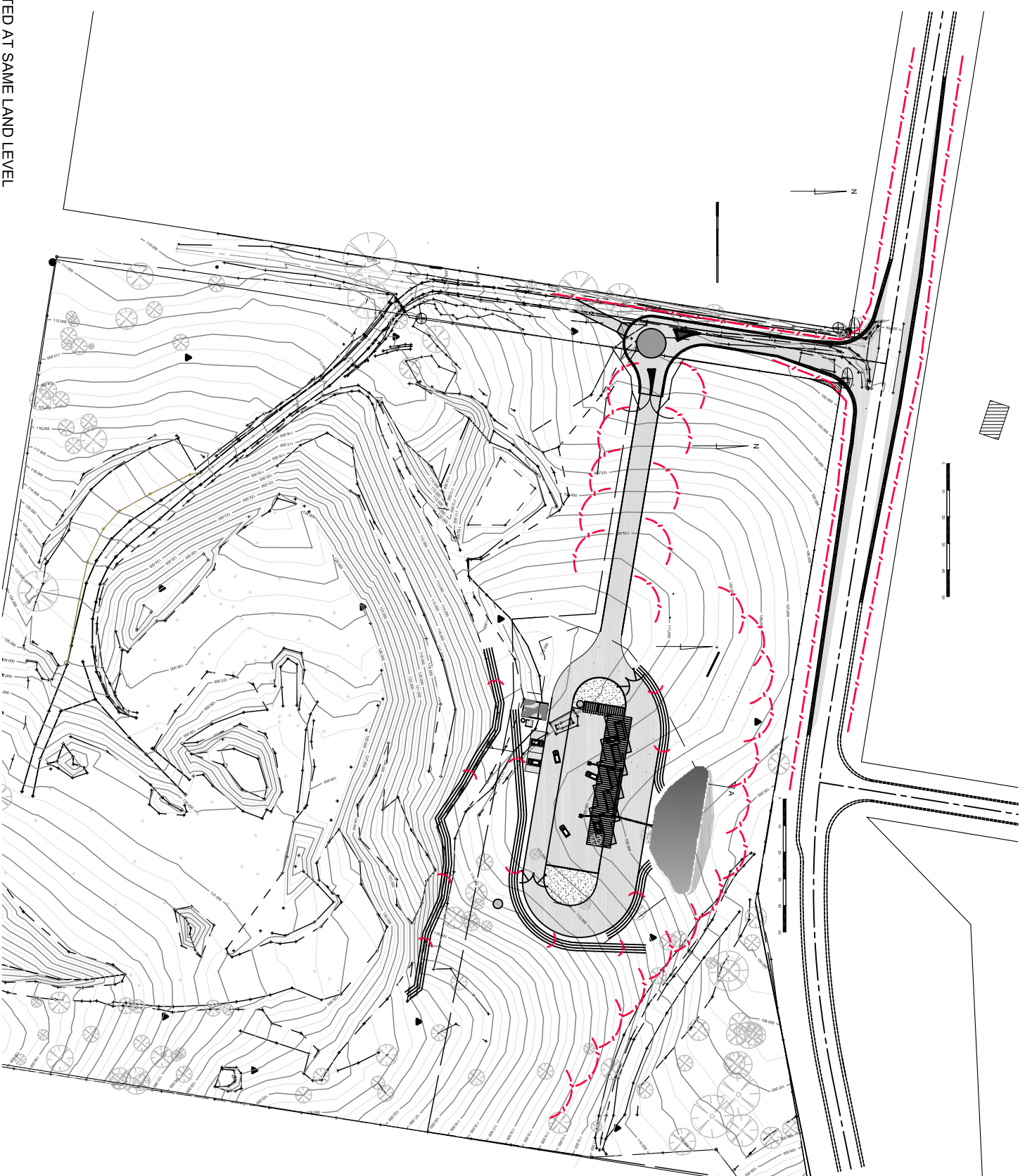
SEDIMENTATION AND EROSION CONTROL PLAN (NTS)
